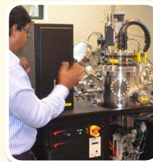
The **LCVD and Thin Films Laboratory** includes PLD/ MBE 2300 equipment and a state-of-the-art pulsed laser deposition system that is capable of depositing atomically thin layers of most solid materials onto any substrate material up to 50mm in diameter.
