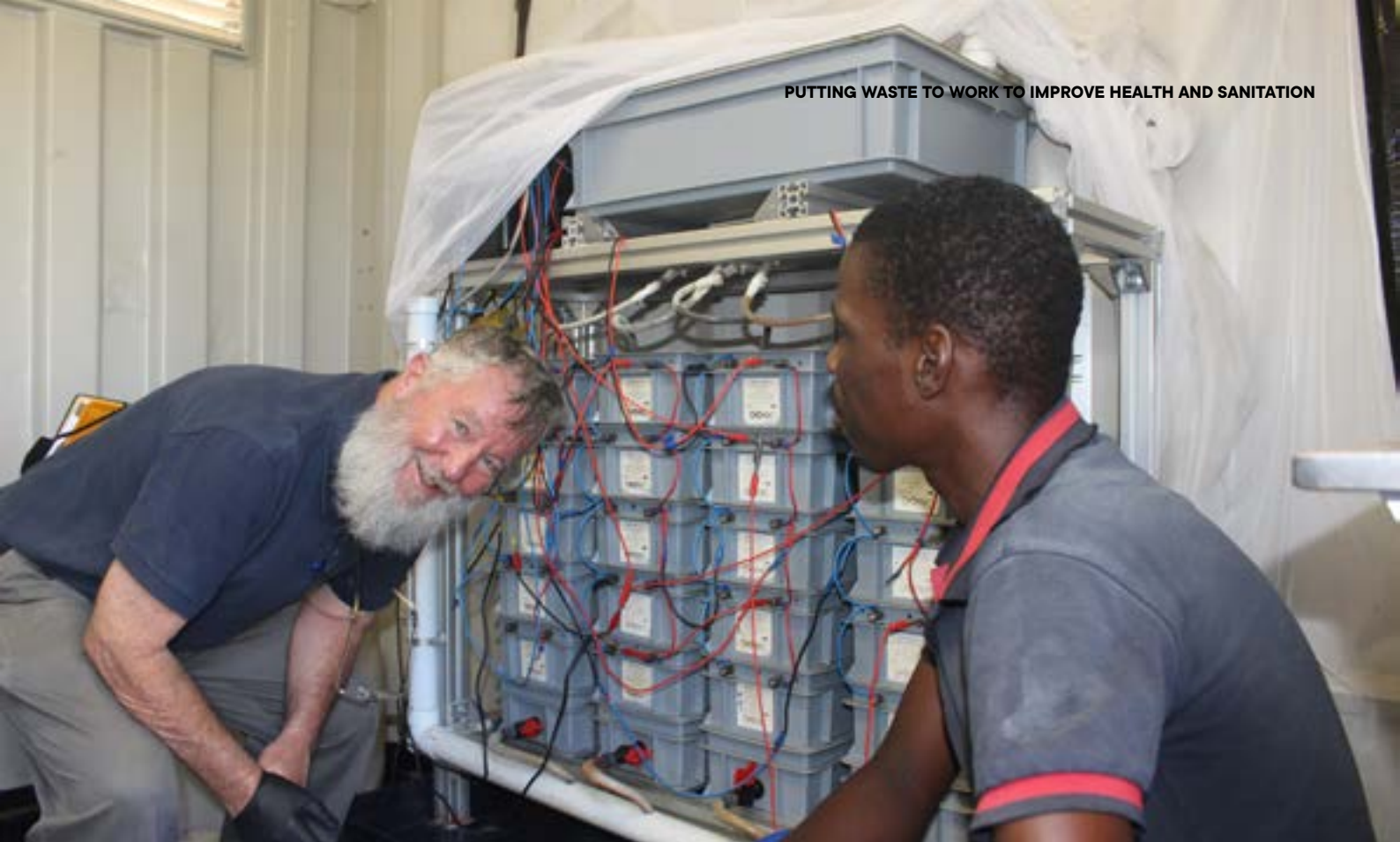
Professor Chris Buckley and community liaison officer, Mr Nelson Khumalo inspect the business end of the ‘uricity’ prototype power plant, where urine was collected from a communal ablution block at a Durban informal settlement.
